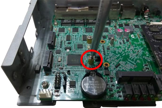
2. Align the notches of the M.2 card with the socket keys in the slot. Tilt the end of the gold fingers down while carefully inserting the card into the slot.
