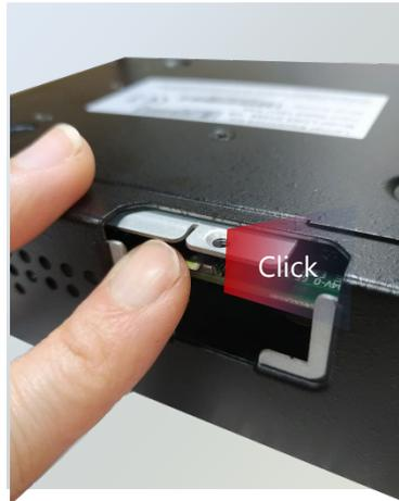
The SIM socket supports push-push mechanism, allowing the SIM card ejection to be as easy as one push. To remove the card, push the card with your fingertip or a paperclip to have it bounce out automatically.
