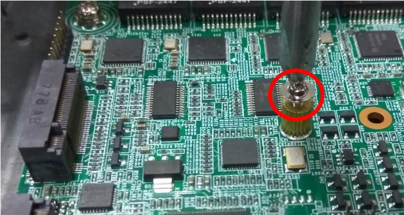
2. Align the notch of the M.2 card with the socket key in the slot. Tilt the end of the gold fingers down while carefully inserting the card into the slot.
