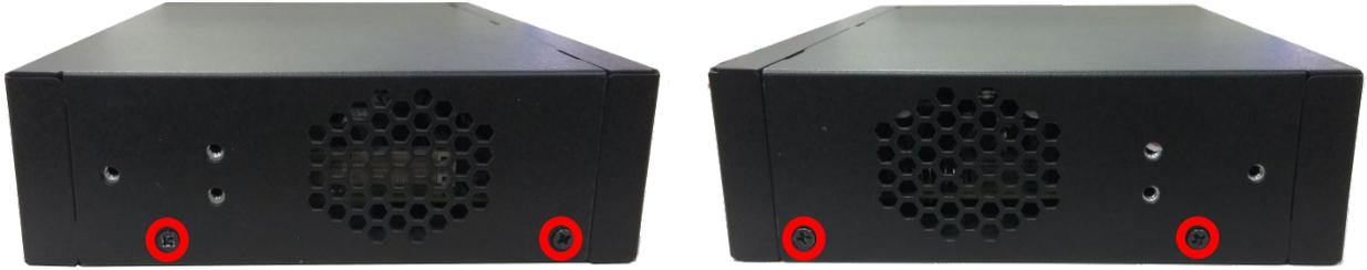
2. Loosen the screw that fixes the SIM Slot cover, and then pull open the bottom panel.
