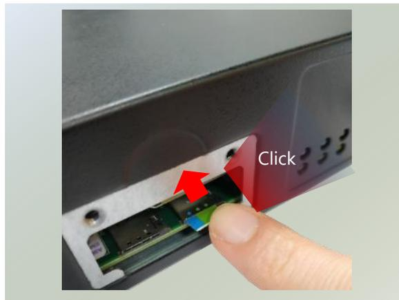
3. To remove the SIM card, use your fingertip to push it a little to have the card automatically ejected.
