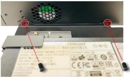
5. Secure the adapter's cable onto the adapter holder.
