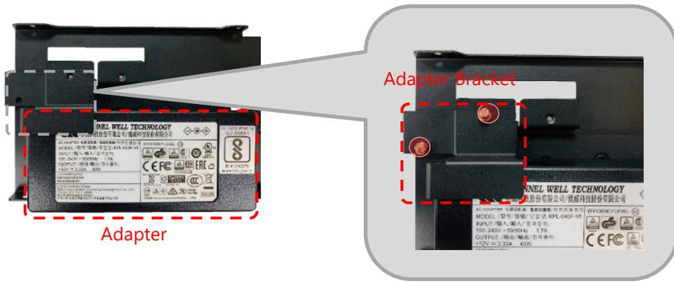
4. Attach the adapter holder to the left side of system and secure it with 2 screws (Screw A)
