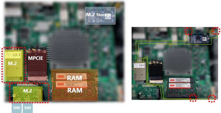
2. Align the notches of the M.2 card with the socket keys in the slot. Tilt the end of the gold fingers down while carefully inserting the card into the slot.
