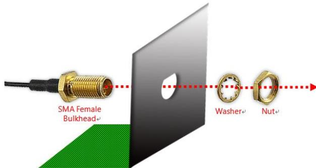
2. From outside the panel, attach the Washer and Nut, and tighten the Nut using an SMA Torque Wrench.
