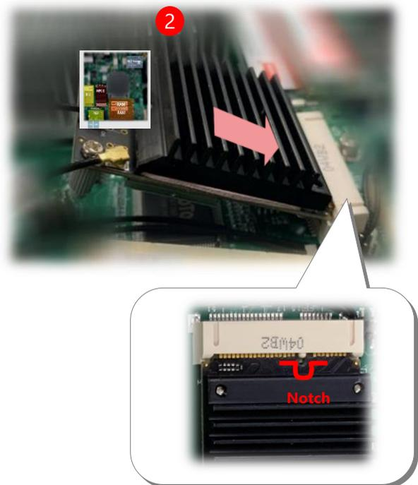
3. Fix the module with the screw provided in the accessory pack.
