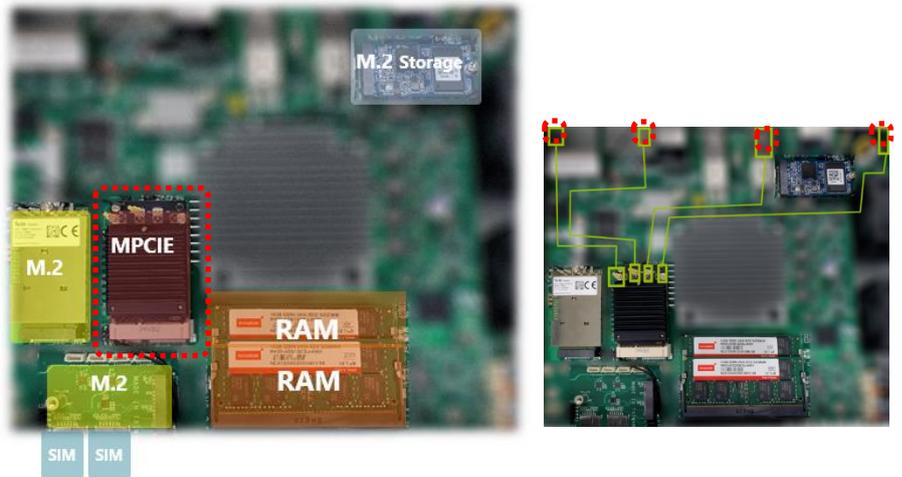
2. Align the notches of the card with the socket keys in the slot. Tilt the end of gold fingers down while carefully inserting the card into the slot.
