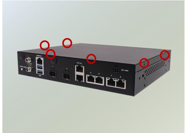
2. Pull open the chassis and lift it up to remove.
