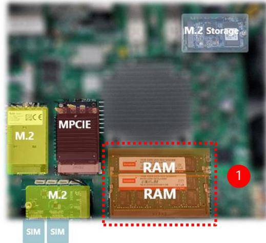
2. Align the notch of the module with the socket key in the slot. Tilt the end of the golden fingers down while carefully inserting the card into the slot.
