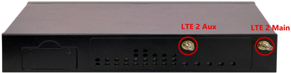
**C. Antenna Placement Optimization for 1x 5G module:**
