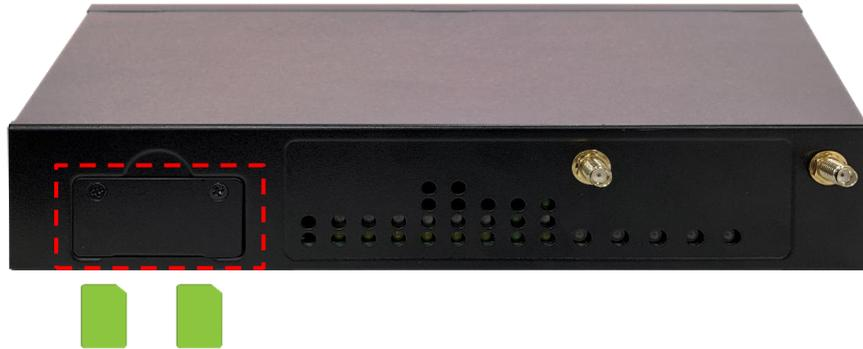
1. Loosen the two screws that secure the SIM slot cover and remove the slot cover. With the angled corner facing inward, push the SIM card all the way in until it clicks into place.
