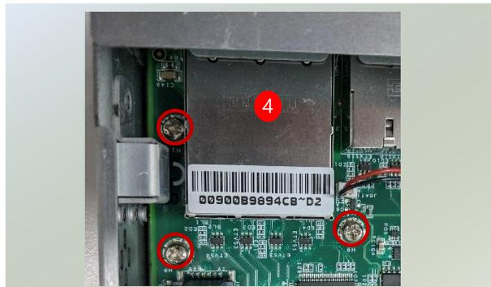
5. Replace the three (3) screws with the spacer standoff pillar studs.
