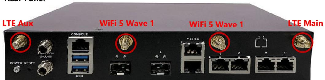
**H. Antenna Placement Optimization for 1x LTE and 1x WiFi 5 (802.11ac Wave 2):**
